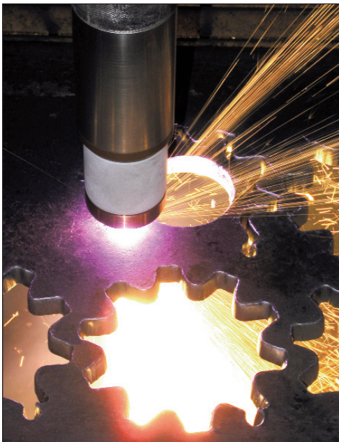
Plasma can be manipulated to cut through metals at high velocity.
