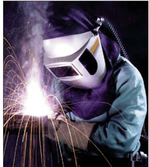
A welding helmet and flame retardant clothing protect a welder from sparks, heat and ultraviolet rays.
